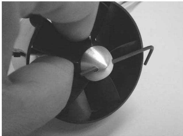
6. Screw the spinner onto the threaded shaft and tighten while holding the spinner in place making sure it is secure. Use an L-wrench or something similar to help tighten the spinner.
