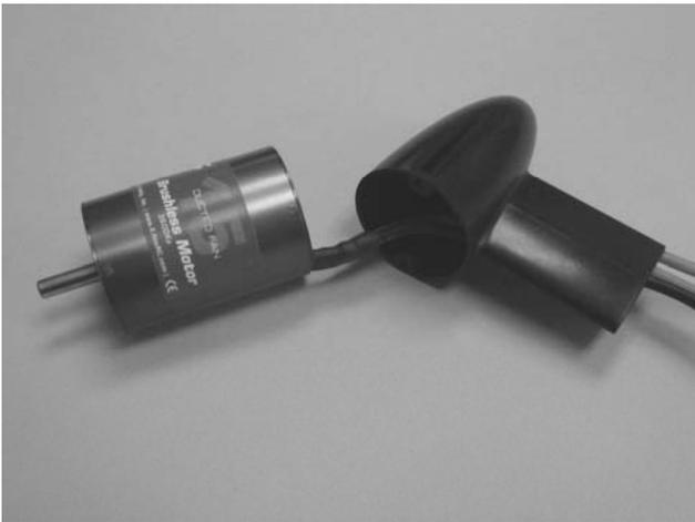
1. Slide the motor wires into the center body fairing as shown.
