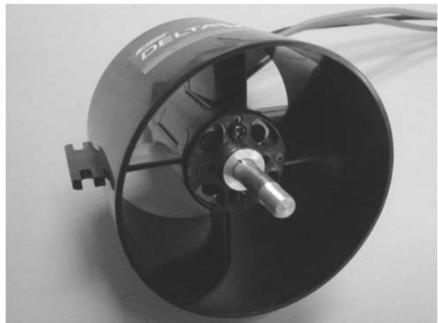
4. Slide the threaded shaft and collet onto the shaft of the motor as far as it will go.
