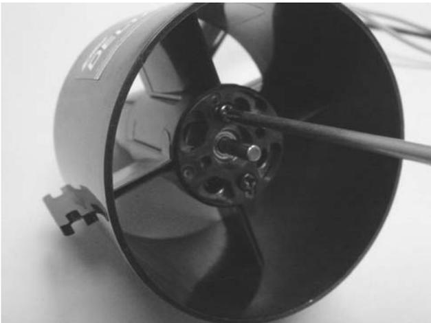
3. Attach the motor to the fan unit using the two 3mm x 5mm screws provided.
