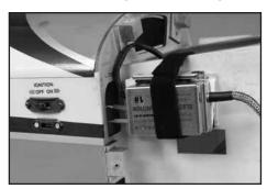
6. Install the ignition module and battery securely in the airplane forward area. It is recommended that a thin piece of foam rubber is placed between the module and the mounting surface and that Velcro® strap is used to hold the module in place.
