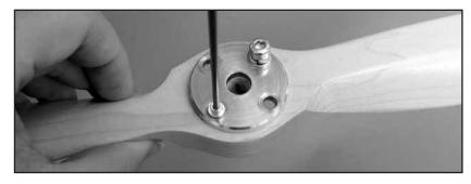
7. Use one of the 5x40mm SHCS with 5mm lock washers and 5mm flat washers to align the propeller washer on the propeller and use the Dead Center Hole Locator to mark position of the remaining holes.
