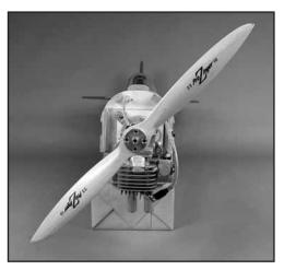
4. Place the propeller on the crankshaft at the 1 o'clock position.
