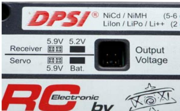
Selecting full battery voltage for the servos (receiver stays at 5.9V):
