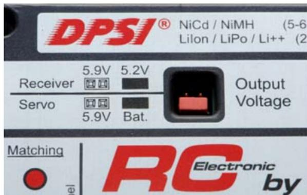
The positions of the jumpers on their multi-pin connectors and their corresponding output voltage are printed onto the housing of the **DPSI RV Mini**. Because a **DPSI RV Mini** should be mounted vibration-less the jumpers can not fall out.
