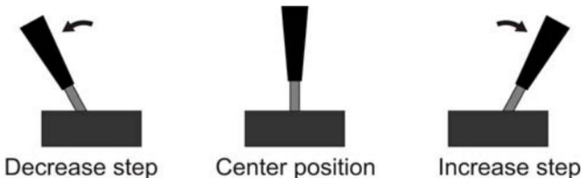
Holding the stick in its end position the steps increase or decrease automatically after 2.5 seconds. This serves for quicker settings.
