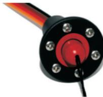
Switching (On/Off) occurs with an external magnet, which resides in a funnel-shaped opening of the switch actuator when in off (SPS turned off). The magnet holds itself due to its magnetism. By pulling easily on the magnet (or key ring) the magnet is removed from the opening and the
