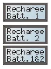
Low voltage battery 1. If the battery is discharged down to about 60% - 70%, this text is displayed. At the same time the error code is beeped by the buzzer every 7 seconds (3 short and one long beep).
