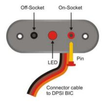
Turning the **DPSI BIC** on is done by putting the pin into the red socket. Putting the pin into the black socket, turns the **DPSI BIC** off.
