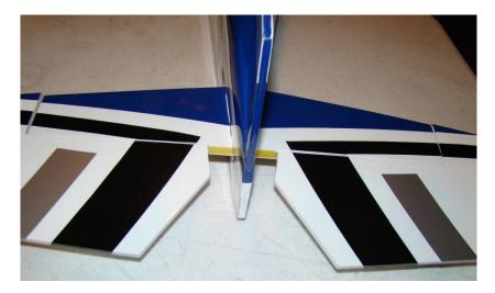
Adjust elevators left-to-right to align with stabilizer. You may notice some twist of the elevator assembly. This will not affect flight performance. If you wish to remove any twist for cosmetic reasons, have a helper twist the assembly slightly the opposite way, and shrink out the resulting covering wrinkles with a heat gun. This will remove any twist.
