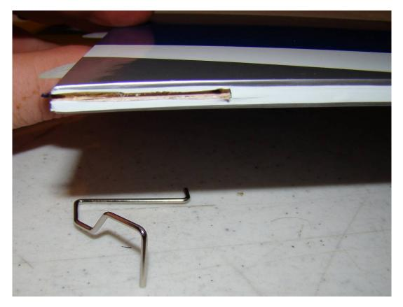
Use small drill bit, small screwdriver, or end of tailwheel wire to make a hole in the rudder at the appropriate spot and insert tailwheel wire into rudder. Check location against manual photo, and if the wire is in the correct location, remove and put a generous amount of medium CA glue into slot. Install wire and allow to cure.
