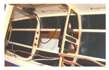
Install your receiver onto the receiver mount in the fuselage as shown using Velcro or a Zip-tie.
