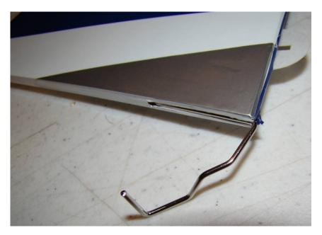
Install rudder onto fuselage, sliding hinges into slots in rear of fuselage and vertical stabilizer. Check alignment of bottom of rudder and fuselage as shown. Drip two large drops of thin CA glue onto each hinge. Allow to cure.
