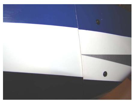
Remove cowl, place a drop of thin CA glue into each hole in the fuselage, allow to cure, and re-install cowl with 4 small wood screws as shown.
