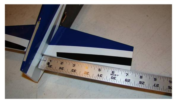
Insert horizontal stabilizer (note the color scheme on top). Use a ruler to square the stabilizer side to side as shown.
