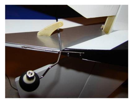
Pushrod connectors – The pushrod connectors attach to the servo arm with a nut, as shown. When you install these pushrod connectors, do not tighten the nut all the way, the connector must be free to rotate. Place a drop of medium CA on the end of the nut and apply CA accelerator to lock it to the threads. You must lock the nuts on your servo connectors, otherwise the nuts will vibrate loose and your plane will crash.
