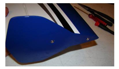
Attach wings to fuselage with nylon wing screws. NOTE – the carbon wing tube is designed to be removable, and is not meant to be glued in place.
