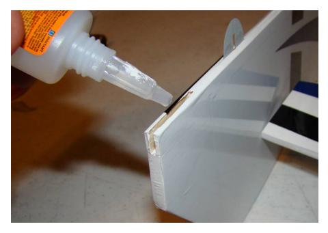
Install elevator half with joiner rod onto horizontal stabilizer, sliding hinges into slots in stabilizer DO NOT GLUE HINGES YET. Apply a generous amount of medium CA into joiner slot on second elevator.
