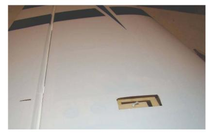
Remove covering over servo opening and aileron control horn slot as shown.
