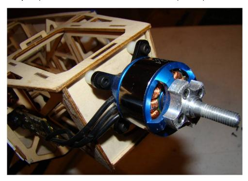
Attach your speed controller to the side of the motor box with plastic Zip-ties or Velcro.
