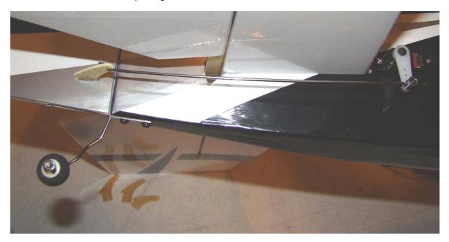
Use the longest pushrod in your kit for the rudder. Install as shown
