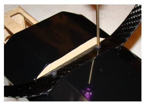
Attach landing gear cover plate. For permanent installation, use medium CA glue. To be able to easily access landing gear screws, use clear tape to attach plate.
