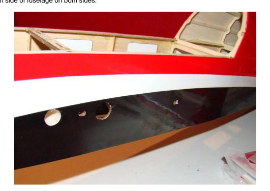
Remove one square of covering from the fuselage bottom behind the wing as shown, for a cooling vent.
