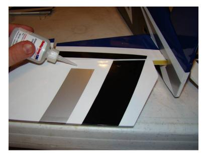
Remove covering over slot in bottom of rudder as shown.
