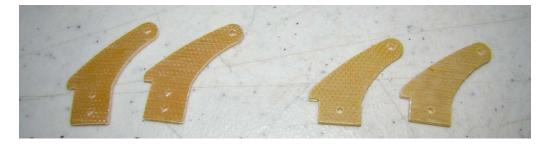
Remove the covering over the slot in the rudder on the RIGHT side as shown, apply a generous amount of medium CA into the slot and onto the bottom of the control horn. Insert horn into slot fully as shown and allow to cure.
