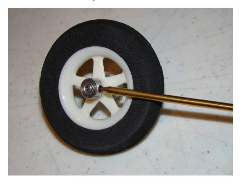
Place wheel and axle assembly inside wheel pant. Attach wheel/pant assembly to carbon landing gear as shown using locking nut. NOTE: The locking nut will be difficult to tighten since it is a locking design. Use a pliers to hold the wheel collar and a nut driver or wrench to turn the nut.
