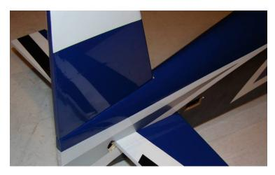
Drop a few drops of thin CA onto the elevator joiner rod at the factory joint of elevator and rod. Allow to soak in for a few minutes, then wipe off excess.
