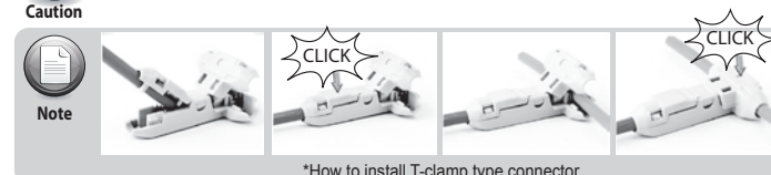
*How to install T-clamp type connector
