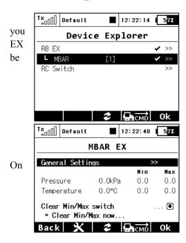
MBar EX sensor can be easily configured via any DC/DS transmitter. If switch the paired receiver to the EX Bus mode and you connect the MBar to its Ext. port, the device will be detected automatically and then might configured in the menu *Model*  $\rightarrow$  *Device Explorer*:
