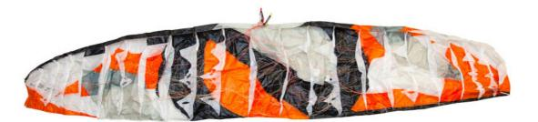
Bring the wing's endpoints to the center of the wing. Put the risers at the bottom of the central cells in order not to mix the bridle and avoid any overflowing.
