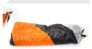
Then, bend the wing in two taking care of not folding the stabilizing rushes. Then insert the wing in its carry bag.
