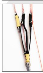
The speedbar bridle has to be set on A lines . In the normal flight position, no strenght has to be applied.
