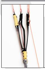
The speedbar bridle has to be set on A lines. In the normal flight position, no strenght has to be applied.
