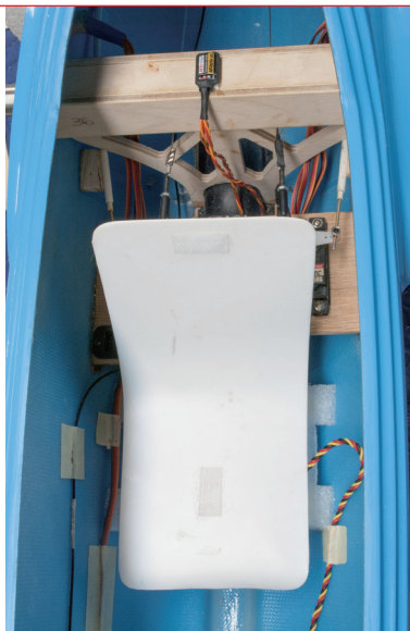
The pilot's seat was fabricated out of polystyrene plastic. The pilot hides the receiver. The vario is fastened to the wing jointer box with Velcro tape.
