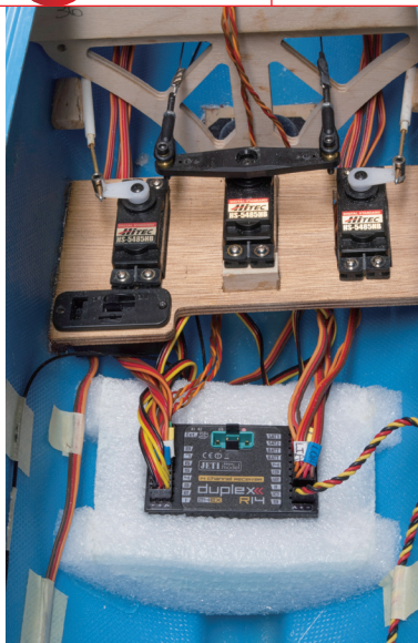
A JETI Duplex R14 channel receiver provides independent control adjustment to all 11 servos. A JETI vario is also used in the XLF-207 ARF.
