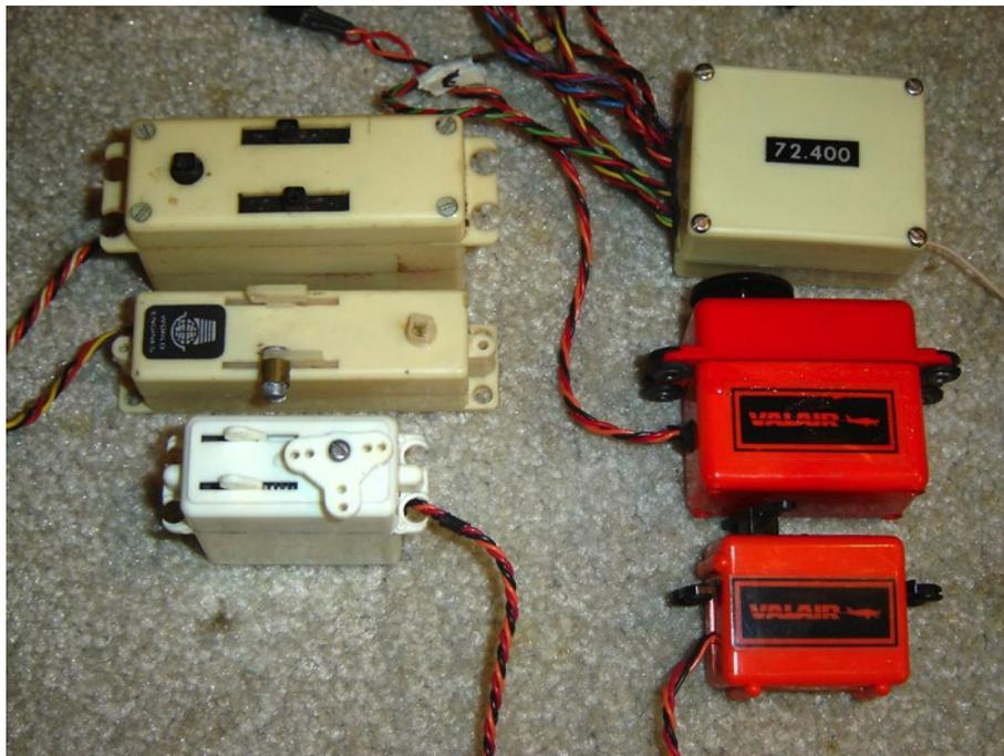
*Upper: The World Engines receiver is at the top and is cube shaped for easier installation in the model. The Valair servos are standard size with good power and very robust gears. These are the most powerful servos I've seen that didn't use rare earth magnets in the servo motors.*
