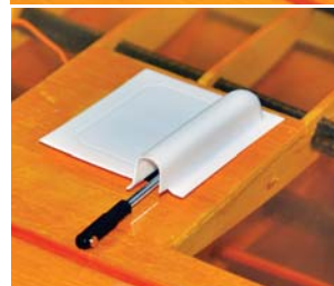
A Spektrum A3030 servo is glued to the servo cover and ready to place into the wing. It was a perfect fit.
