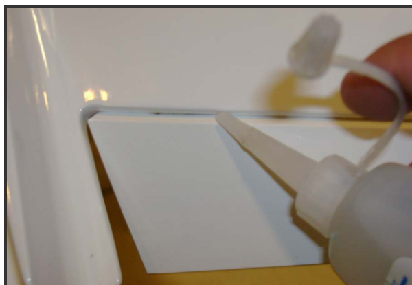
Bond rudder using thin CA adhesive
