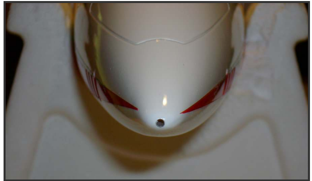
Hole in the nose of the fuselage for the Pitot tube
