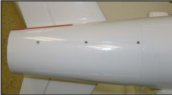
Drill guide pin holes
