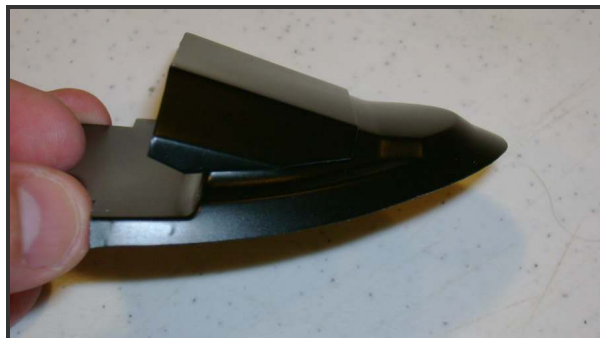
Bond the upper cockpit component to the lower cockpit component with CA adhesive.
