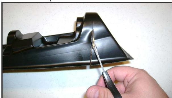
Trim the cockpit to the panel lines
