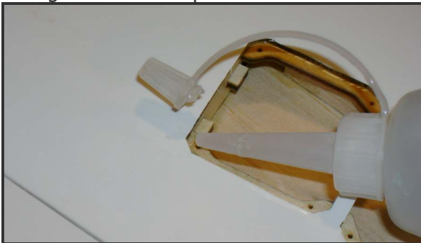
Reinforce screw holes with CA adhesive
