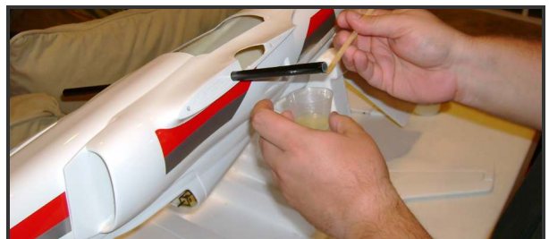
Apply adhesive to the fuselage and wing tube
