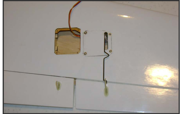
Completed aileron control rod
