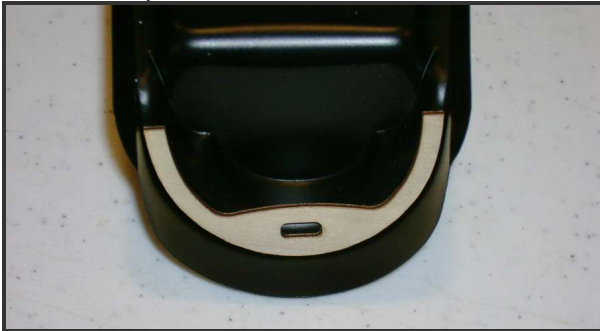
Bond the latch plate to the cockpit
