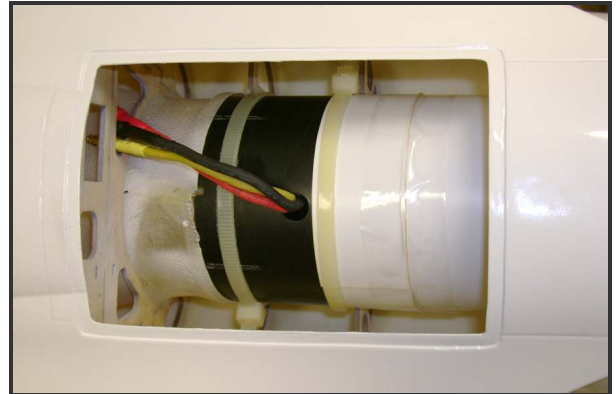
Fan and thrust duct assembly completed
