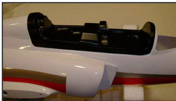
Dry fit the cockpit and make any adjustments
