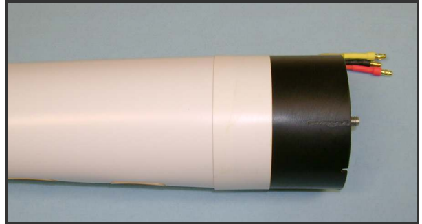
Test fit the thrust duct in fan shroud and EDF unit
