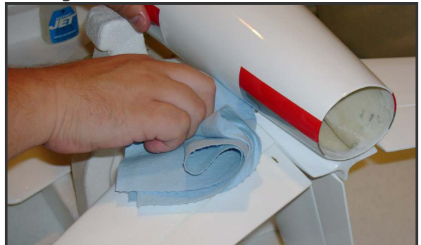
Clean any excess adhesive using a rag with rubbing alcohol
