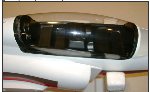
Bond the canopy to the cockpit using canopy glue
