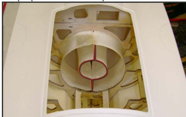
Area where ducts should be trimmed to create rotor clearance when using non SAPAC EDF units
