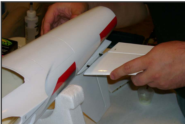
Slide the horizontal stabilizer into position
