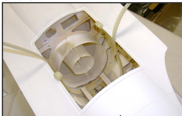
Zip ties in position, note opposite orientation
