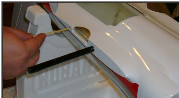
Apply adhesive inside the locating pin holes
