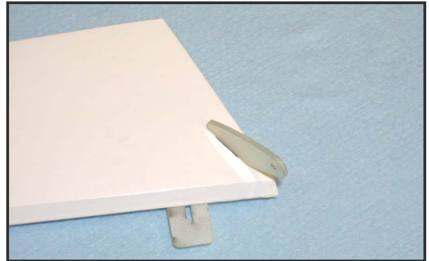
Dry fit the control horn
