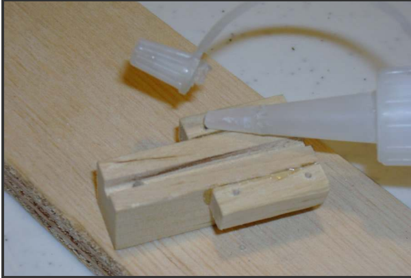
Reinforce holes with thin CA adhesive
