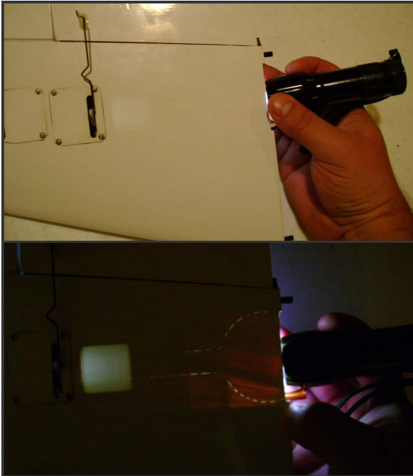
Locate the cutout for the retractable landing gear
