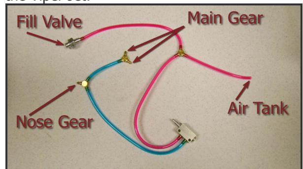
Actuator valve with air lines; blue for gear and red for tank and fill valve
