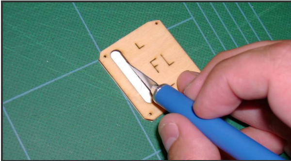
Remove covering from servo arm slots
