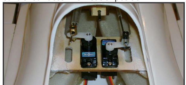
Completed servo installation
