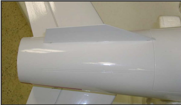
Bond the fins with 5-minute epoxy
