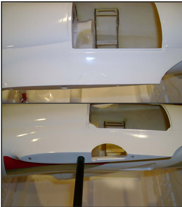
If you are using retracts, cut openings for gear clearance
