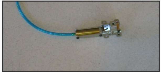
Attach air lines to retract unit
