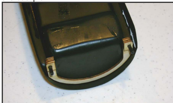
Bond the front pin assembly to the cockpit
