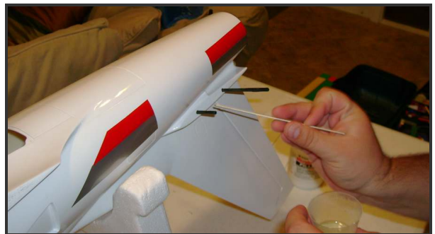
Apply adhesive to the fuselage and to the stabilizer tubes
