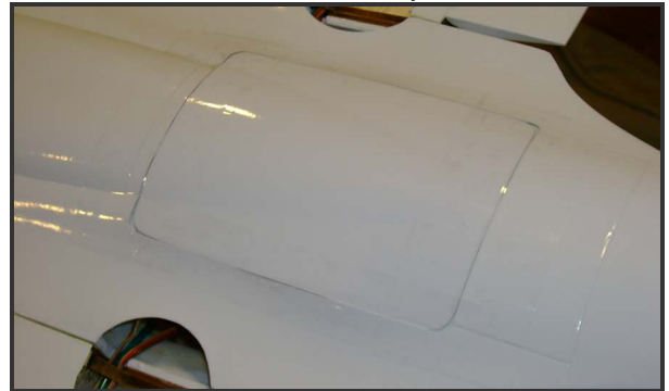
Attach the fan access hatch cover with tape
