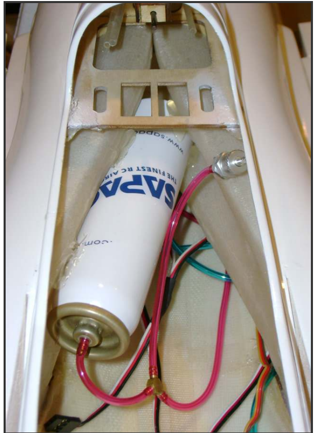
Air tank mounted in location
