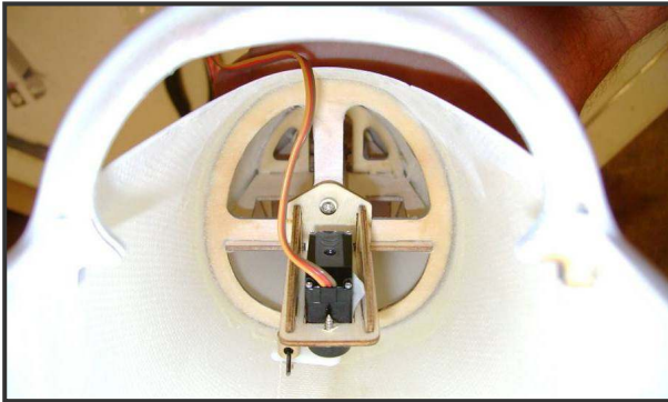
Nose gear mount in position and attached
