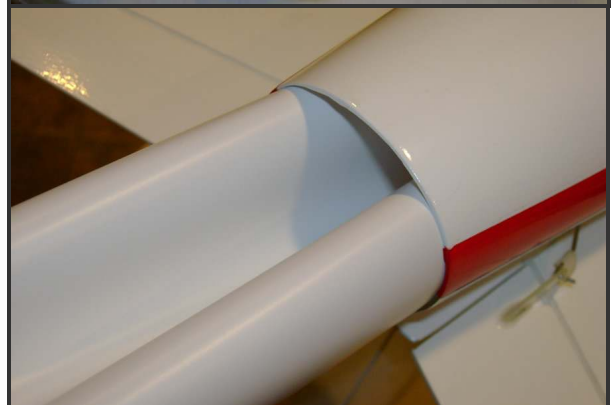
Thrust duct folded into a U shape for insertion through the tail of the airplane
