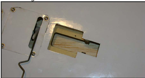
Main gear slot cut into wing
