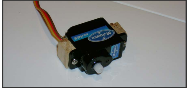
Servo mounting posts screwed to servos
