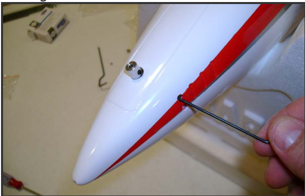
Tighten the inside set screw of the long collet
