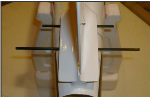
Stabilizer mounting tube locations
