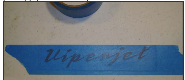
Place a piece of low tack tape on the decal
