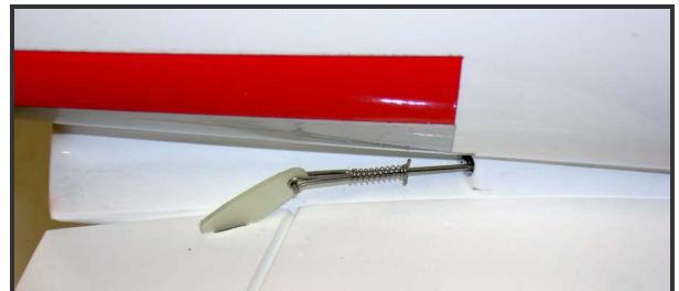
Control rods installed on the tail surfaces
