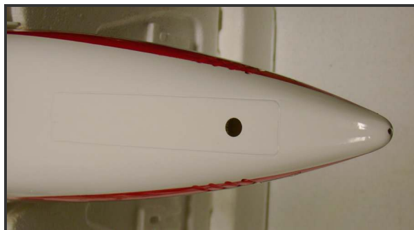
Hole reamed to size to fit the long collet
