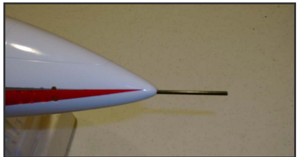
Pitot tube bonded in position
