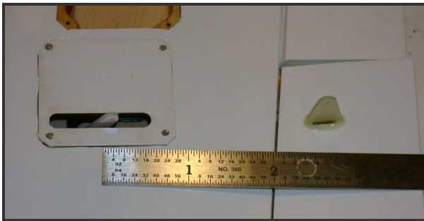
Dry fit servo and measure control rod
