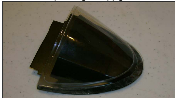
Bond the canopy to the cockpit using canopy glue
