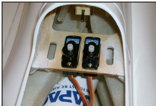
Elevator and rudder servos mounted in position
