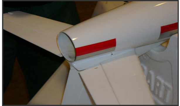
Horizontal stabilizer in its final position
