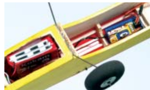
A Kokam 3S 1020mAh Li-Poly pack and Hitec Electron receiver fit comfortably in the Angelis.
