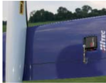
The Hitec HS-125 aileron servos are perfect for the Micro Flash, but the covers do not quite fit. You can smooth the airflow across the servo bays with clear packing tape.
