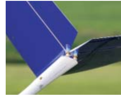
The V-tail only uses elevator control, so a single pushrod, split at the end makes for a clean and straightforward installation.
