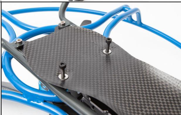
Perform the same operation for the lower part, but this time with a 3mm drill. Then use 2 CHC M3-10 screws and lock nuts for fixing.
