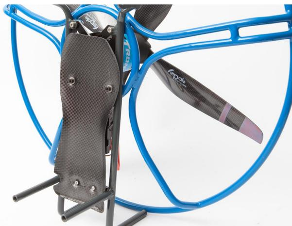
First remove the two lower M4 screws holding the arch to the chassis. Position the carbon plate and drill it with a 4mm drill bit. Once done, replace the M4 screws.
