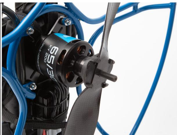
Place the second propeller. Mount the washer and then the clamping nut.
