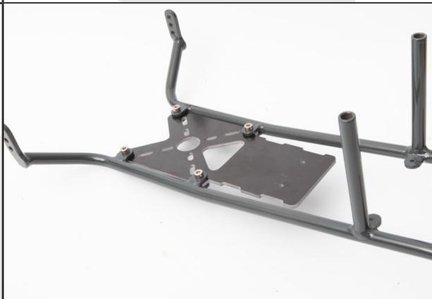
Mount the 2nd plate using 2 CHC 3-10 screws, M3 washer and M3 lock nuts. Please note that this plate must be behind the fixing bracket.
