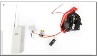
In ejection status, the angle formed has to be -45°. The pin fully release the arming rod.
