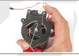
Check that the horn is able to reach this low position during a move. The pin must be place on the second hole of the arming rod.
