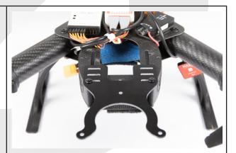
Use 3 CHC M3x10 screws with M3 nuts to attach the tube on the holder.
