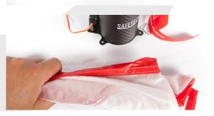
Do several S in the way of the parachute length, as shown on the picture.
