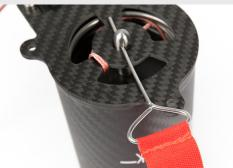
Arrange the horn on the servomotor. Push it up on the highest position. Then place the horn in the position shown on the picture.
