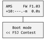
Within this firmware, the telemetry function is disabled (only JETIBOX and SMART-BOX terminal connections remain active). Motor cannot be restarted.
