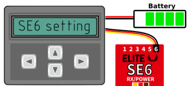
Optional type of connection. The output No.6 must be configured to a "Sensor" option.
