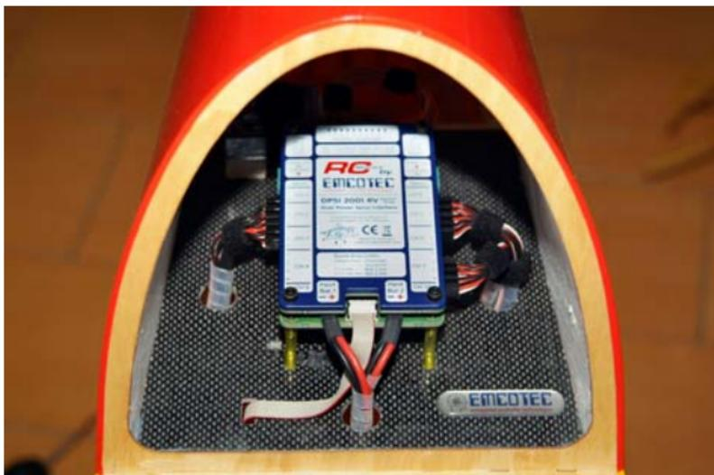
Of course, mounting with screws and short spacers is possible. This is recommended for gliders or jets (models with little vibrations, see photo on page 17).
