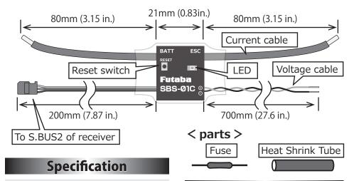
Use: Current sensor Detection item: Current (0A ~ 150A) Voltage (0V ∼ 70V)
