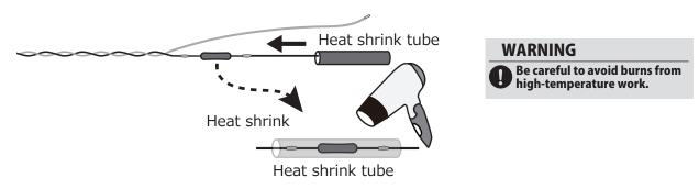
4 The cable should be connected as shown in the diagram below.
