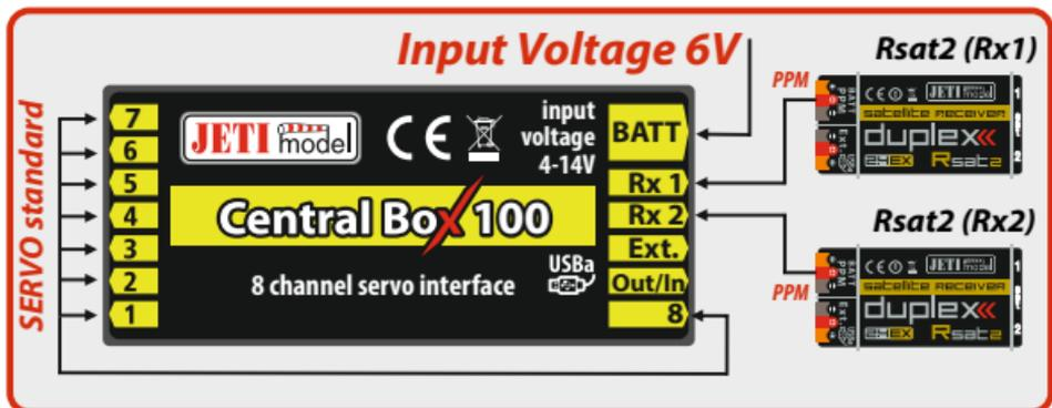
Fig. 5: Example of the Central Box 100 powered for use with standard servos (voltage up to 6V)
