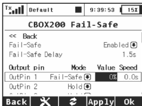
Fig. 16: Device Explorer-Fail Safe
