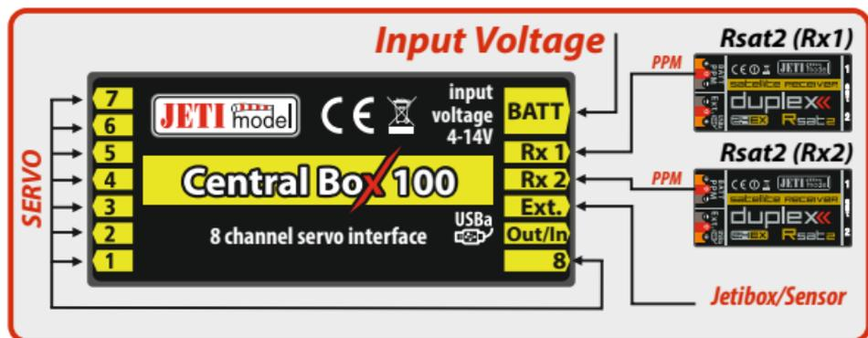
Fig. 11: Block diagram of Central Box 100 connection - EX Bus variant
