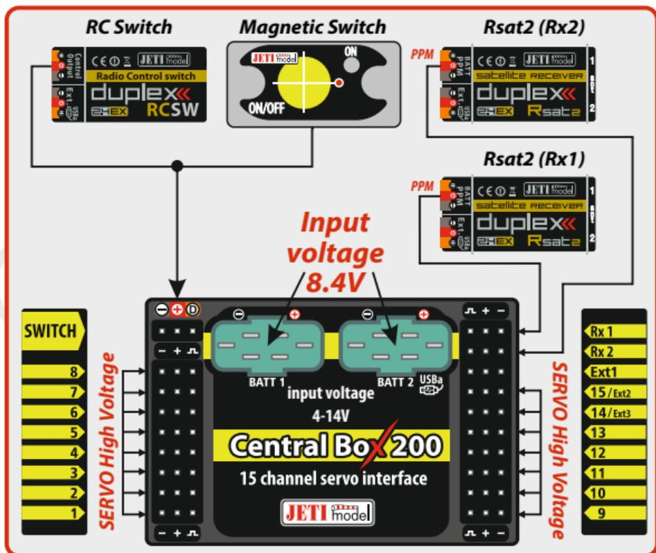
**Fig. 6: Example of the Central Box 200 powered for use with HIGH Voltage servos**
