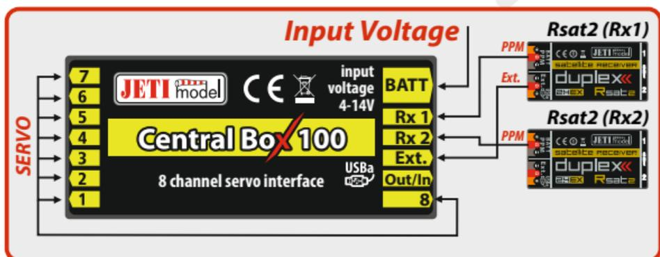
**Fig. 9: Block diagram of Central Box 100 connection - PPM variant**
