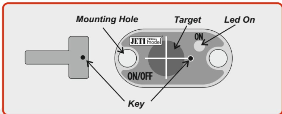
**Fig. 3: Description of magnetic switch and the key**
