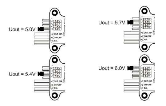
Using the Jeti Box terminal, navigate to the Output (x.x) Volt setting (See section 4.3 SETTING - Configuration Options) and change to your desired value. This can be done in steps of 0.1V independently of the position of the short-circuit/jumper plug.
