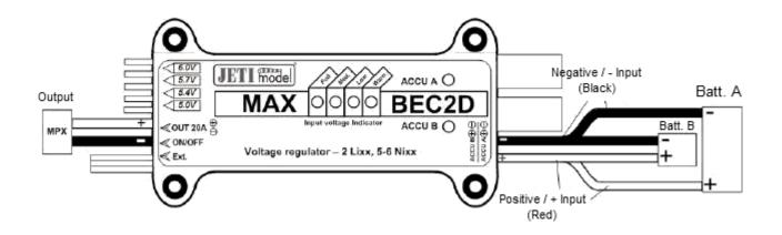
To connect your device(s) to the BEC, either solder your wires (Please use wire of at least 1mm2 diameter or larger, depending on your anticipated load) to the MPX output connector of the BEC or use the Jeti MPX/3xJR cable, available separately. The Duplex EPC receivers, such as the R6 EPC, R8 EPC, R12, R14 and R18 are already fitted with a compatible MPX plug.
