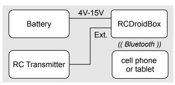
transmitter. The connection is realized using a three-wire cable with a standard servo-connector on both sides. A separate power supply from battery 4V-15V with the correct polarity and voltage needs to be connected to the RCDroidBox battery connector. The final component is the cell phone or tablet running both the operating system Android (2.3.3 or higher) and the RCDroidBox application.
