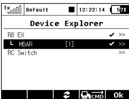
MBar EX sensor can be easily configured via any DC/DS transmitter. If switch the paired receiver to the EX Bus mode and you connect the MBar to its Ext. port, the device will be detected automatically and then might configured in the menu *Model* → *Device Explorer*.
