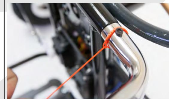
The brake bridle must slide in the ring fixed at the extremity of the arm. Thanks to this type of mounting, the clearance of brakes is multiplied by two. Perform the same operation on the other servomotor.
