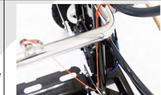
This bridle must be connected directly on the brake bridle of the wing. Once the connection done, cut the surplus of the bridle.
