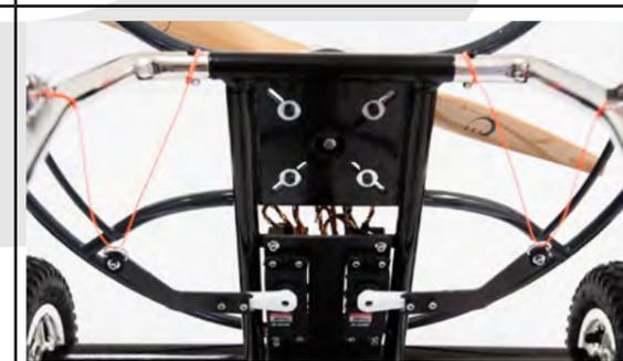
Here is the position of the servomotor with 0 signal (in that case, the remote controller does not include a mixer).
