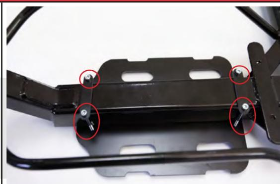
By the mean of a cutter, remove the painting that is in the surface of the trike.
