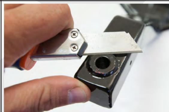
Position the front fork. This one must accomodate without any difficulty. If not, remove by mean of a cutter the painting that is at the other extremity of the passage of the axis.
