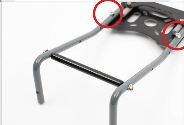
Fit the black bar using 2x CHC M3-12 screws with 2x M3-Small washers.
