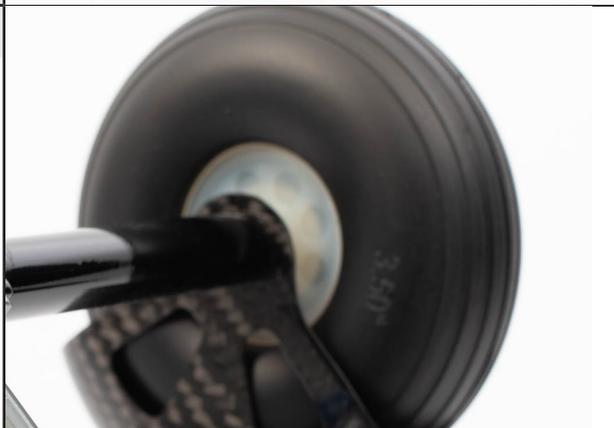
Attach the two side bars to the rear axle using 4x CHC M3-25 screws, 4x M3 locknuts and 8x M3 washers.
