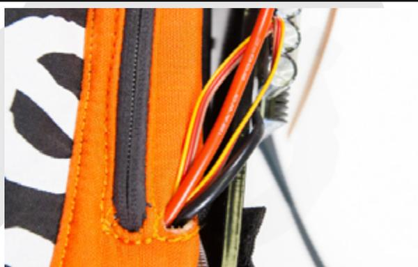
Connect the ESC to the receiver installed inside the pilot.
