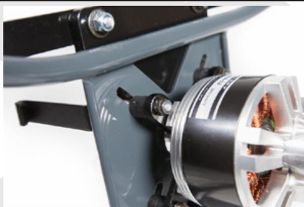
Use 4 screws CHC M4-12 with M4 nuts to fix the ESC on the back of the pilot plate.
