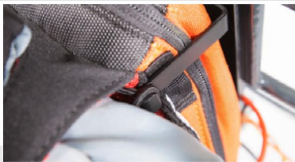
Attach then the elastic on the other edge of the pilot fixation.
