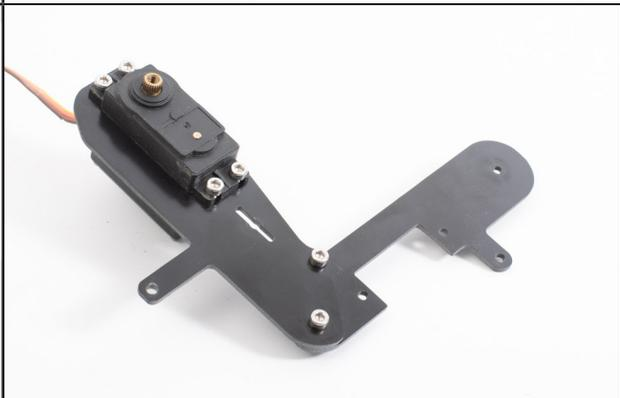
Mount the back part with an M3-8 screw and M3 locknuts
