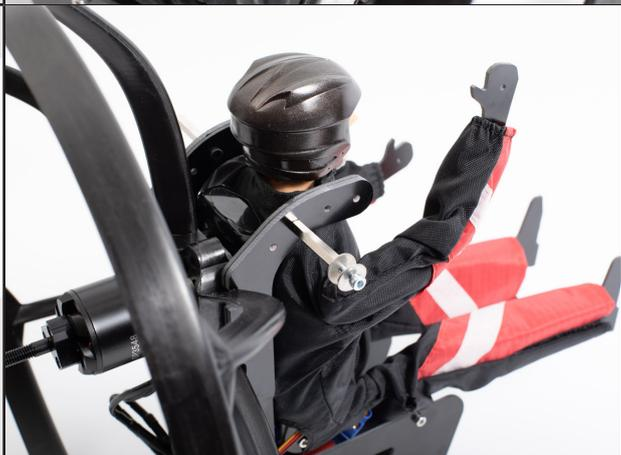
To fix the risers, use 2 M3 large washers with a CHC M3-20 screw
