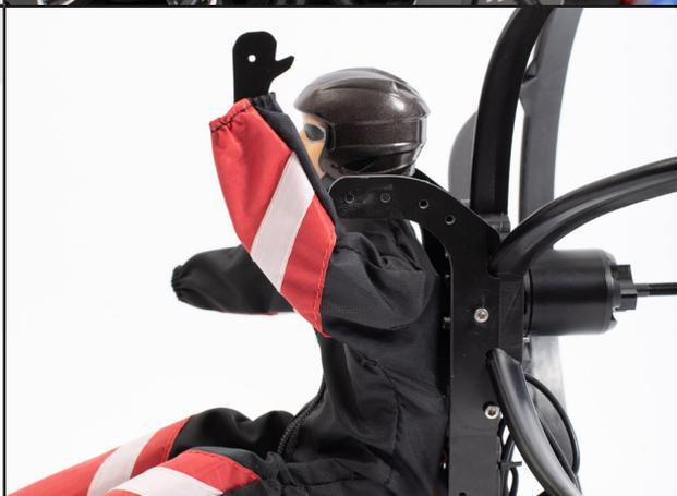
The back of the pilot is designed to accommodate a 3 to 4S 2000 to 2500mAh battery. Insert it to then proceed to the balancing of the chassis
