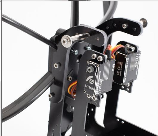
In order to optimize the volume, the mass, the responsiveness of the whole, the servo support kit is designed to accommodate the OPS1715AHV servomotors, both for the arms and for the accelerator part. They are to be mounted on the sides using CHC M3-8 screws and corresponding locknuts.
