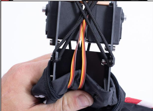
Insert the speed controller cable through the driver's suit (it is preferable to put the receiver there as well)
