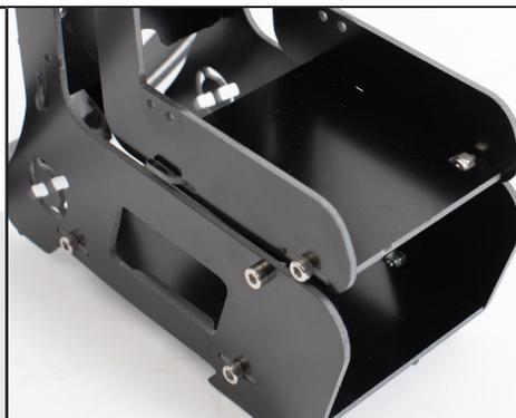
The assembly of the kit follows the same logic as that of the pilot. The sides are mounted with M3-8 screws and M3 locknuts. The vertical fixing is done with two M3-12 screws, and the low fixing with 2x M3-8.
