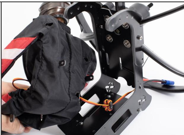
Fix the pilot's legs to the frames using 2 CHC M3-8 screws and M3 locknuts
