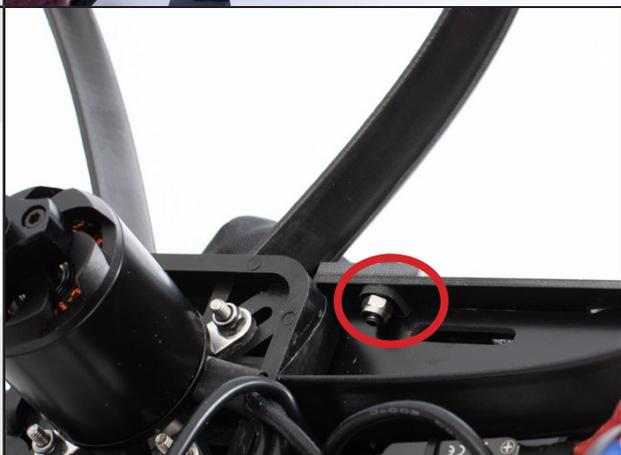
Then fix the arms on the servomotor horn, using 2 Phillips 2x8 screws.
