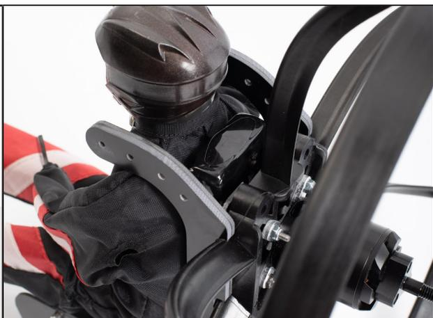
The frame's balance point must be at the anchor point. On this point, the chassis must remain, in working order (ready to fly), horizontal.
