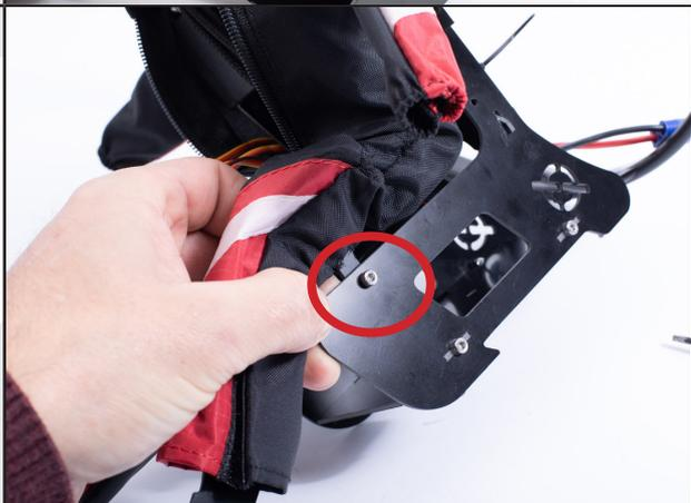
The pilot's back is fixed using CHC M3-10 screws and locknuts.
