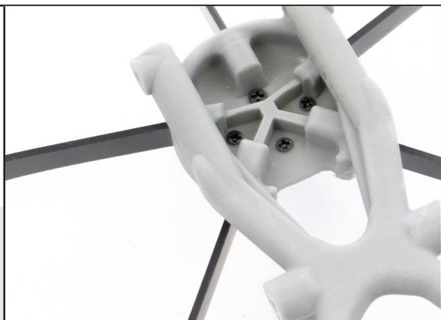
Position the lock plate in GFK, and then the motor. Do not forget to add threadlock on the 4 motor fixing screws. The stays are thus locked.
