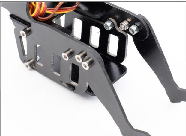
Fit the engine OP1806 propeller mount. It is strongly recommended to use a thread lock for mounting the motor.
