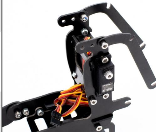
Position 4 CHC 3x8 screws on the back frame. Do not tighten as much as possible, leave a space of 4mm.
