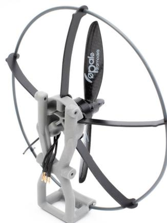
Mount the two back stays using CHC 3x8 screws and locknuts.
