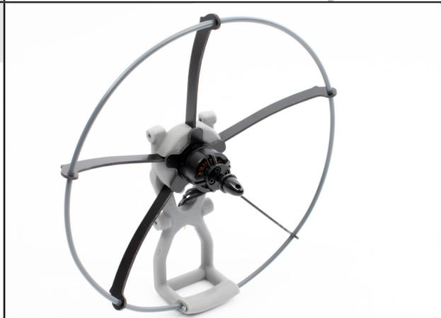
Insert the propeller with the appropriate spacer. The logo on the propeller must be facing forward. It is important to always check the position of the leading edge of the propeller. This one must always be positioned towards the front of the chassis. a reversed propeller will directly result in a lack of power.
