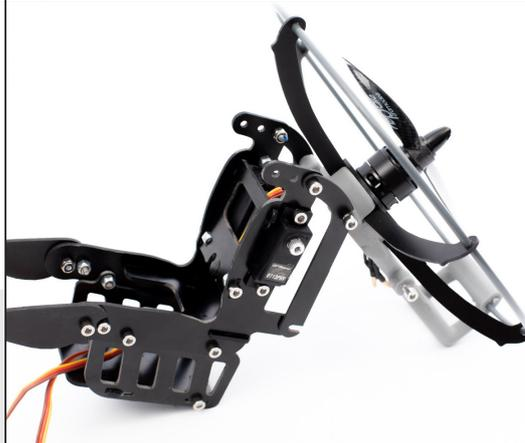
Then fit the bottom part and proceed to the tightening operation of the 4 x 3x8 screws.
