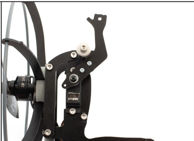
in the low position -100%, the arm must be in this position.
