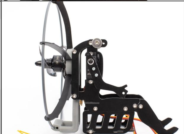
Then mount the two M3-30 spacers on the chassis with a 3x8 CHC.
