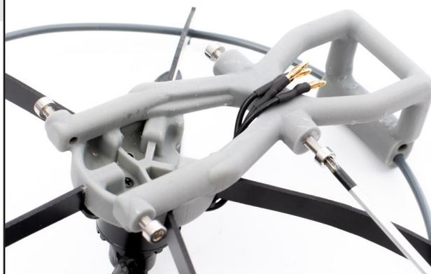
Mount the back frame by the two top screws at first.
