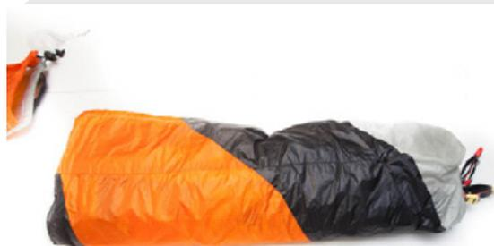
Then, bend the wing in two taking care of not folding the stabilizing rushes. Then insert the wing in its carry bag.
