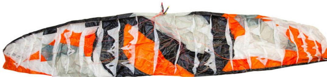
Bring the wing's endpoints to the center of the wing. Put the risers at the bottom of the central cells in order not to mix the bridle and avoid any overflowing.
