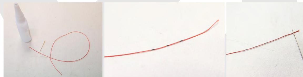
Use a needle to be papered, with a round endpoint and liquid cyanoacrylate glue. To perform the first buckle, put a mark at 4 cm from the endpoint with a marker pen. Then, put 2 another marks with 1cm space between each. Then place the endpoint in the needle's hole.
