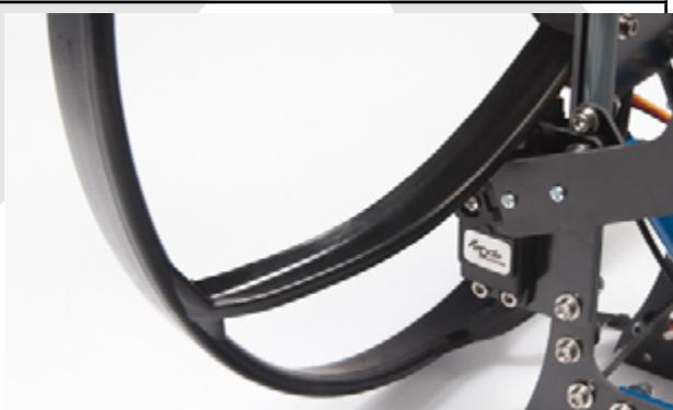
Power up the servomotor, and adjust the mechanical end position with your remote to have the arm in the same position than on the picture shown. The stick of your radio must be in the middle position (which is defined as the highest position in your remote settings).
