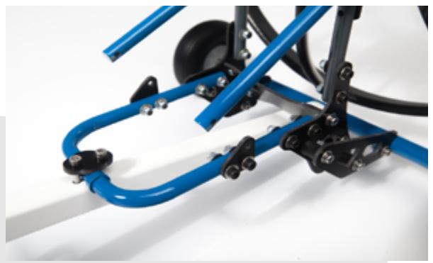
Position the lower plate on the servo holder kit as it is shown on the picture.
