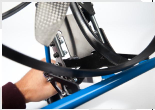
Then tighten the plate with the CHC M3-16 screws removed earlier.
