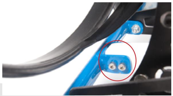
Place the silent blocs with some CHC M3-8 screws, washers and nuts. The silent blocs ensure the mechanical junction between the landing gear and the Backpack. It is necessary to place the 4 silent blocs.
