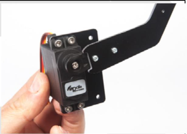
Position the whole thing as shown on the picture and tighten the whole thing with CHC M3-20 screws, washers and nuts.
