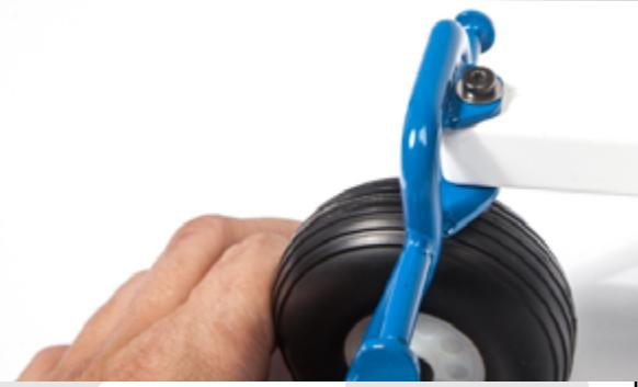
Fix the wheel with 1 x M4x40 screw. Place first the M4 nut, and tight it enough but not too much in order to preserve the wheel rotation on the wheel. Then place the whole thing on the rear axle and tighten the nut against the rear axle. The wheel can move freely. Then do the same with the opposit wheel.
