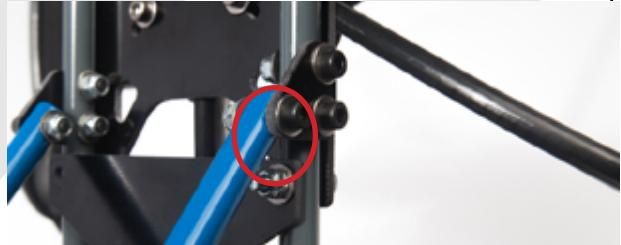
Use the ergots on the vertical plate to maintain the elastic. It will allow to hold the battery in the same position.
