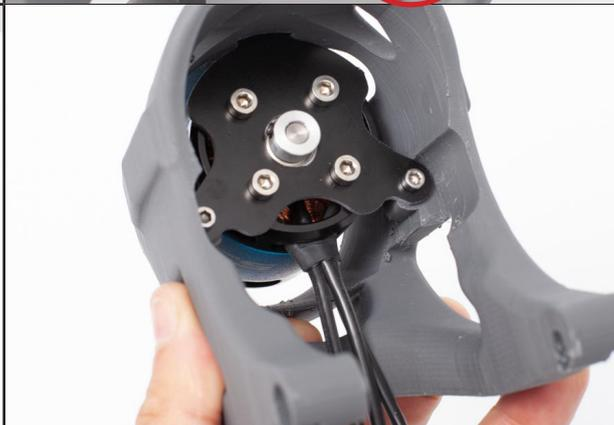
Connect/Solder the speed controller to the motor.
