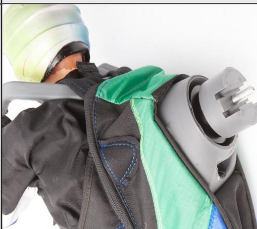
Place the pre-assembled propeller on it
