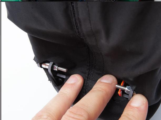
Position the motor support on the two screws
