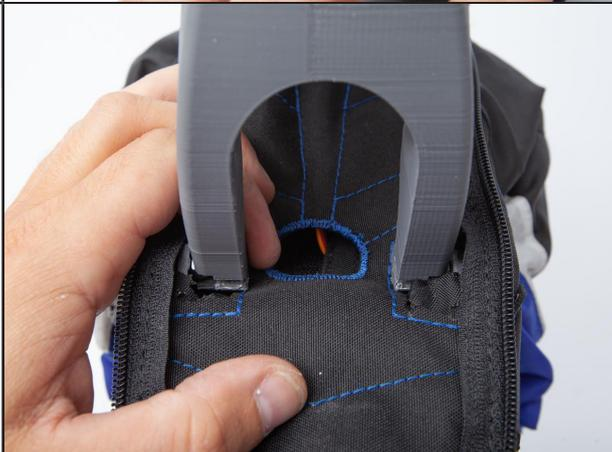
Pass the cables of the ESC through the harness and between the velcro of the pilot's suit
