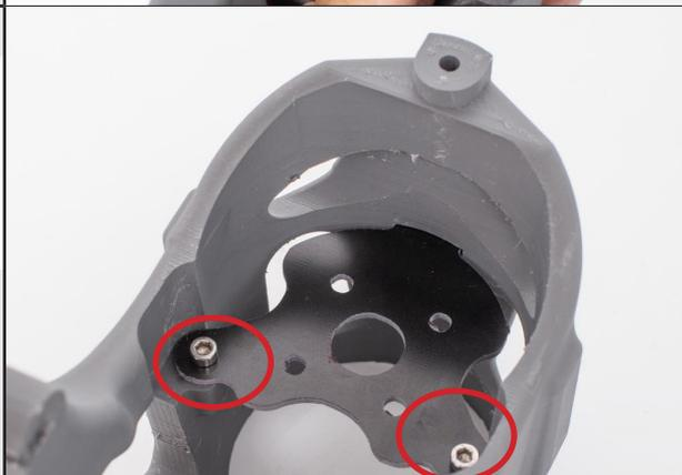
Position the motor and fix it using 4x CHC M4-8
