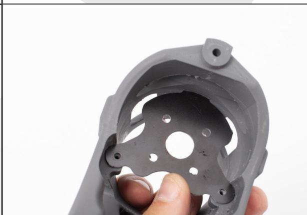
Secure the plate using 2x CHC M3-10
