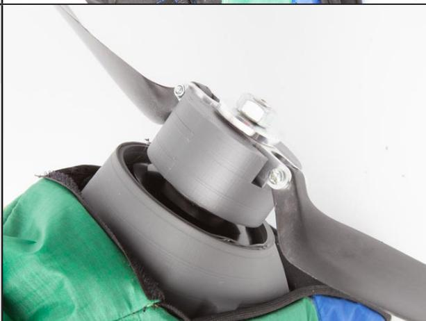
Pass the propeller in the elastic and go up to the hub
