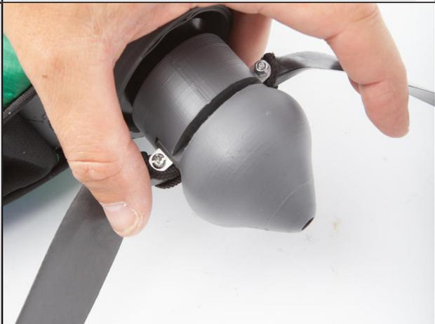
Fix the cone using a CHC M3-10
