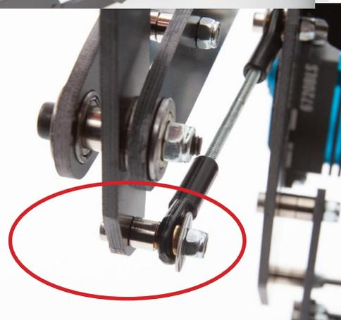
Drill the last hole of the aluminum beam supplied with the OPS4820BLS / OPS6720BLS servomotors using a 3mm drill bit.
