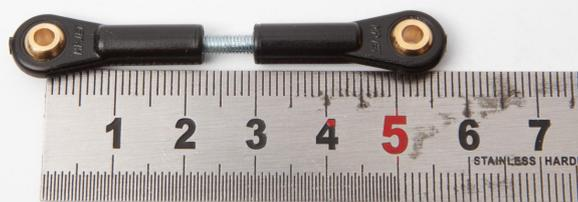
Mount the connecting rod on the servomotor horn using a CHC M3x12, large M3 washer and M3 lock nut. Pay close attention to the direction of assembly, it must imperatively be as shown in the photo. In the opposite arm, there will be a mechanical collision when using the arm.
