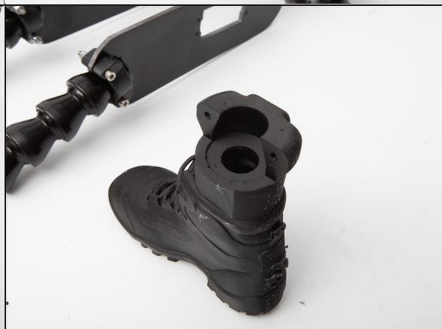
Secure the shoe using 2 CHC M3-25 screws and M3 lock nuts.
