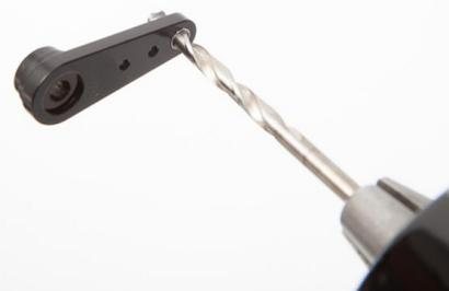
using a servo tester or a Jetibox, position the servo motor halfway (i.e. 1,500ms) Then put the servo arm perpendicular to it.
