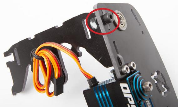
Position the bearing supports. The bearings must be in opposition with the sides (to be checked with the shoulder of the bearing)
