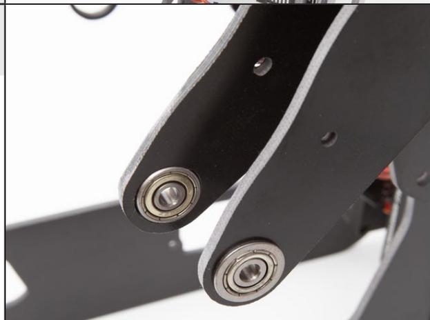
The assembly of the forearm is done with an M4-25. Between the forearm and the bearing an M4 spacer. Then another M4 washer between the forearm and the arm. Finally, use an M4 lock nut
