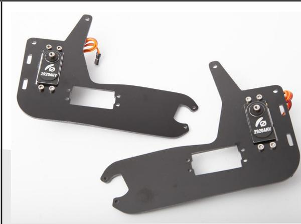
Assembly of the lower back plate using 2x CHC M3x8 screws and lock nuts.
