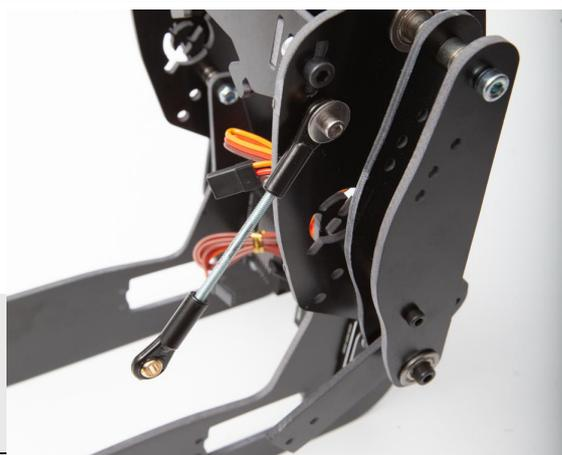
Fixing the connecting rod on the forearm is done with an M3x16 screw, an M3 spacer, a large M3 washer and M3 lock nut. Same for the opposite side
