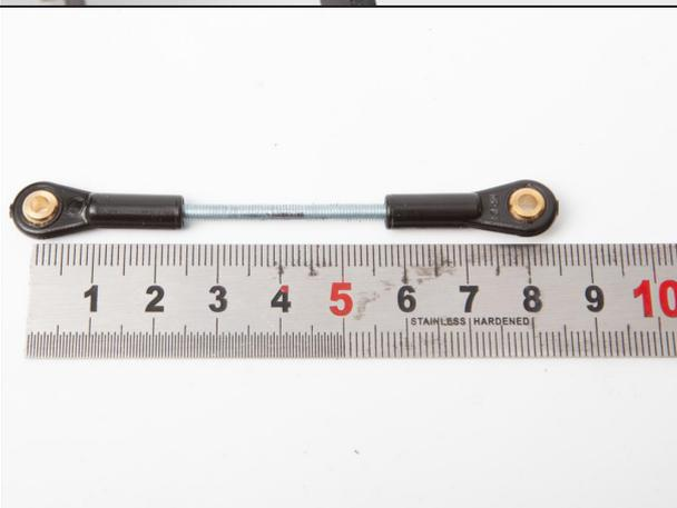
Attach the connecting rod to the driver's trunk using a CHC M3-16, large M3 washer and M3 lock nuts.
