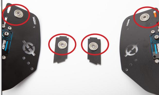
Mount the back plate. Secure it using a CHC M4x12 screw and M4 lock nut
