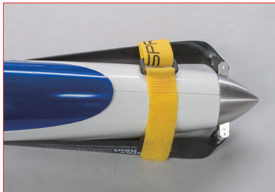
Esprit's hook-n-loop propeller retainer is a nice add-on to your order because it will keep the propeller out of harm's way during transit and storage.
