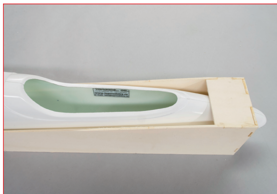
This plywood jig makes cutting the nose off the fuselage to turn the glider into an LMR machine easy and quick to do.
