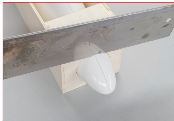
You'll want to use a sharp Zona-type saw to cut the nose off the fuselage. During the cut it must be held tightly against the jig.
