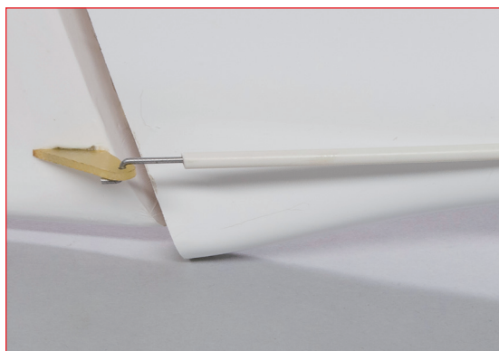
The piano wire pushrod uses a Z-bend at the rudder end. It runs through a sheath to the servos, so there is no slop in this control linkage.
