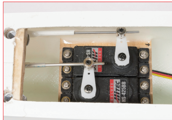
The elevator and rudder installation in the fuselage could not be easier to do. Adjustments are quick and simple too by way of easy connectors.
