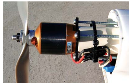
The improvised motor mount extension for the AXI 4130 is lightweight, quite solid, inexpensive and easy to adjust.
